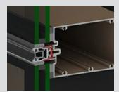
Thermally broken glass support fins protected with anodised aluminium cap to protect from intensive UV degredation.
