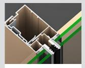
200mm long extruded aluminium retention brackets at mid span and 200mm up from the bottom reduces the risk of mullions seperating.
