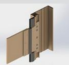
The sun fin bracket is thermally isolated from the mullion, bracket will vary depending on sun fin design
